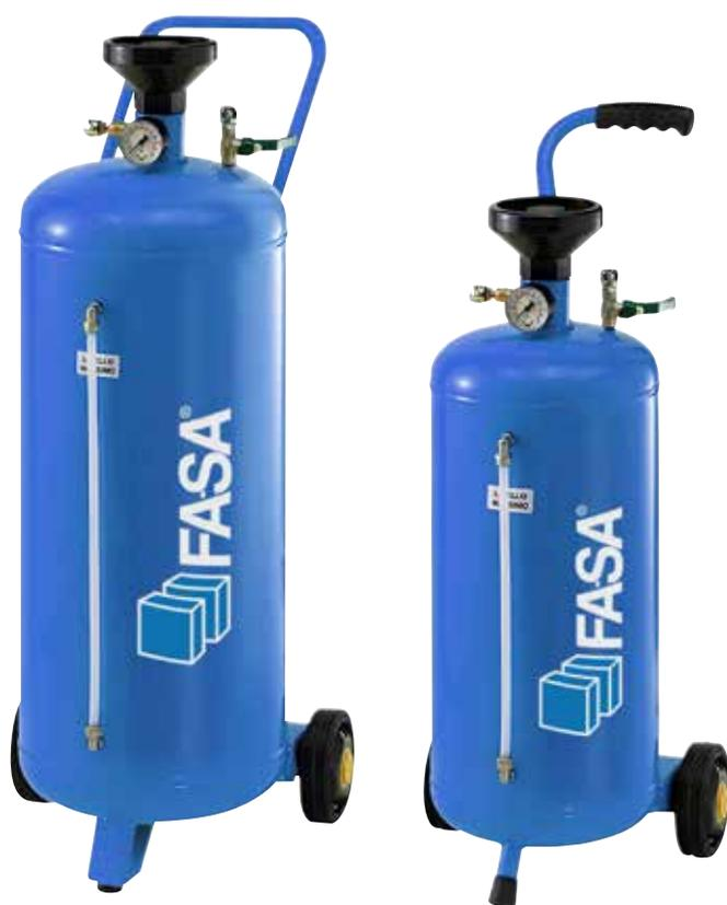
**Spray:** Pneumatic charge sprayers need to be connected to an air compressor to charge the tank and allow the product vaporization without the connection to the air compressor. They work at high-pressures and so they use capacious steel or stainless steel tanks to allow a greater working autonomy.
