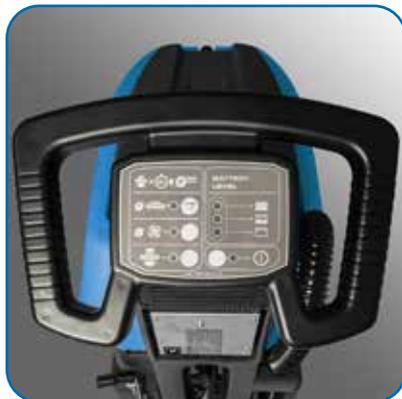
Protection against overloads, battery discharge abuse (DC only) and undesired run. Convenient one switch maintenance over the brush. Eco Energy setting for extensive working time and extremely quiet operations (DC only). Accessible on-
