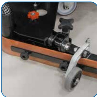
Strong mechanical control levers for heavy duty use. Large size drain hose for a fast emptying and a better cleaning of the recovery tank. Quick fitting battery charger plug.
