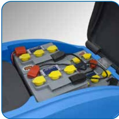
Easy access to battery and vacuum motor compartment, without using tools. Large capacity shock and acid proof polyethylene tanks (88 l) avoid frequent refilling and idle time. 4 x 6V -180 Ah C5 batteries
