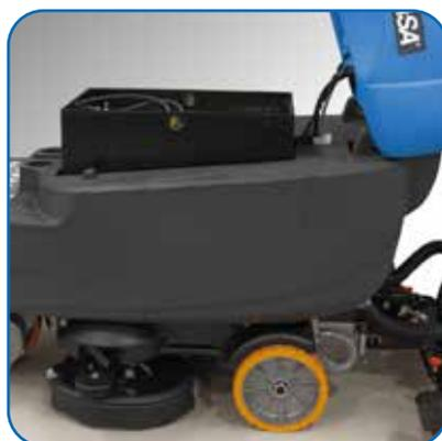
by thermal breakers. 80 kg of continuous brush plate pressure with Self Leveling System to strongly and deeply removing any kind of dirt on any kind of floor. Strong oil-proof polyurethane wheels. 500 Ah C5 battery box allowing continuous working time
